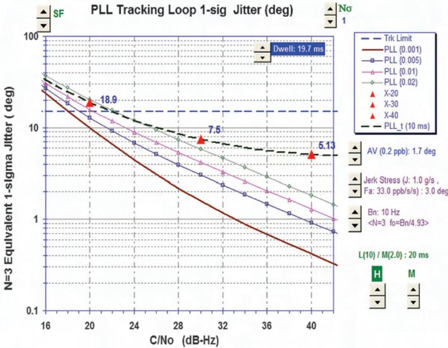
**FIGURE 1** Phase lock loop tracking error as a function of GPS signal carrier-to-noise density. The curves illustrate the effects of four different predetection integration intervals (PDIs) from 1 to 20 milliseconds without a jerk stress and for the 10-millisecond PDI case when the loop undergoes a 1.0-g-per-second jerk stress. In each case, the dwell is 20 milliseconds.
