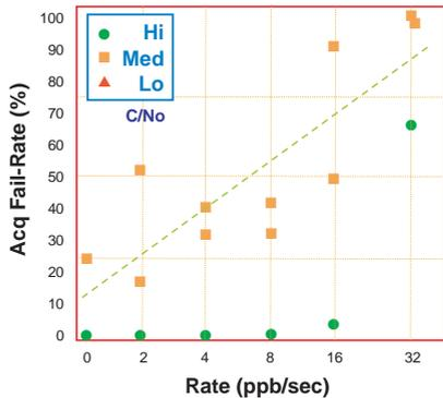
▲ **FIGURE 6** GPS receiver acquisition failure rate in response to varying accelerations of up to 32 parts per billion per second or approximately 1 g (as simulated with a ramp function with a varying rate) for low (less than 25 dB-Hz), medium (25–32 dB-Hz), and high (greater than 32 dB-Hz) C/N<sub>0</sub> values.
