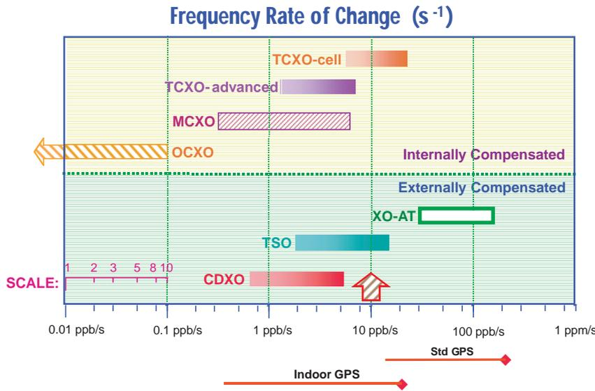
**▲ FIGURE 3** Temperature-gradient performance of different types of crystal oscillator varies widely. TCXO: temperature-compensated; MCXO: microcomputer-controlled; OVCXO: oven-controlled; XO: uncompensated; TSO: temperaturing sensing; CDXO: calibrated dual crystal oscillators.
