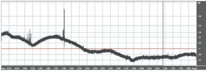
**▲ FIGURE 5** An example of microjumps in a temperature-compensated crystal oscillator following a cold soak. The vertical scale is signal voltage into the oscillator in dB. The horizontal scale is time in hours and minutes.
