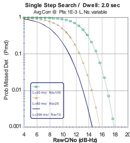
**▲ FIGURE 2B** The probability of the missed detection of weak GPS signals as a function of carrier-to-noise density. The dwell period (L × Ns) was held fixed at 2 seconds, and the predetection integration interval (L) varied from 20 to 200 milliseconds.
