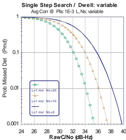
**▲ FIGURE 2A** The probability of the missed detection of strong GPS signals as a function of carrier-to-noise density. The response for three noncoherent summation or dwell periods of 5, 10, and 20 milliseconds is illustrated. In each case, the predetection integration interval (L) is 1 millisecond. The dwell period is L, and Ns is the number of noncoherent samples.
